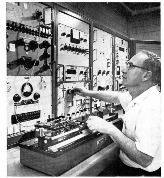
A KELVIN BRIDGE is used by John Ingram to calibrate resistance. The shop is a Sandia standards station for calibrating and certifying electrical and electronic instruments.
